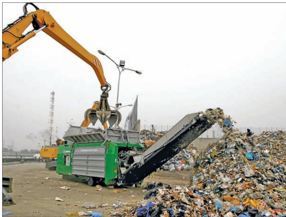
The Komptech Terminator mobile single-shaft shredder processes all types of waste. The amount of waste Americans generated in 2010 rose by 6.2 million tons, the U.S. EPA said.
